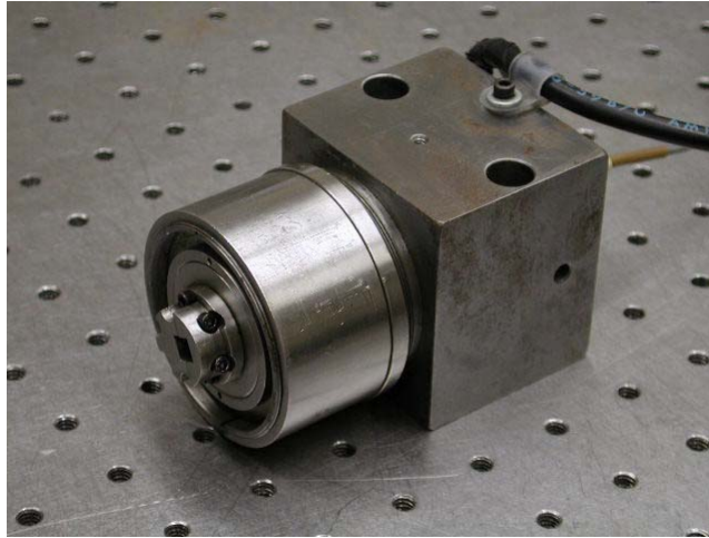
Figure 1: Piezo-based FTS servo developed by NC state researchers (courtesy of NCSU)
