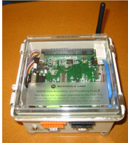
Figure 13: Wireless Data Acquisition Node developed by Motorola and Los Alamos National Laboratory
