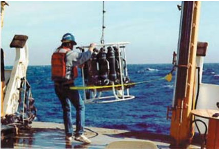
Retrieving the CTD which collects information on water conductivity and temperature at different depths
