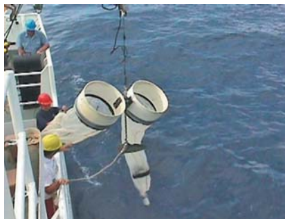
Bongo net is deployed to collect plankton
