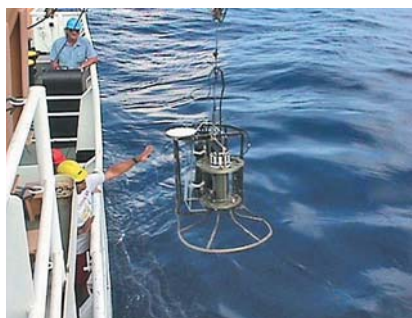
CTD is deployed to take oceanographic measurements
