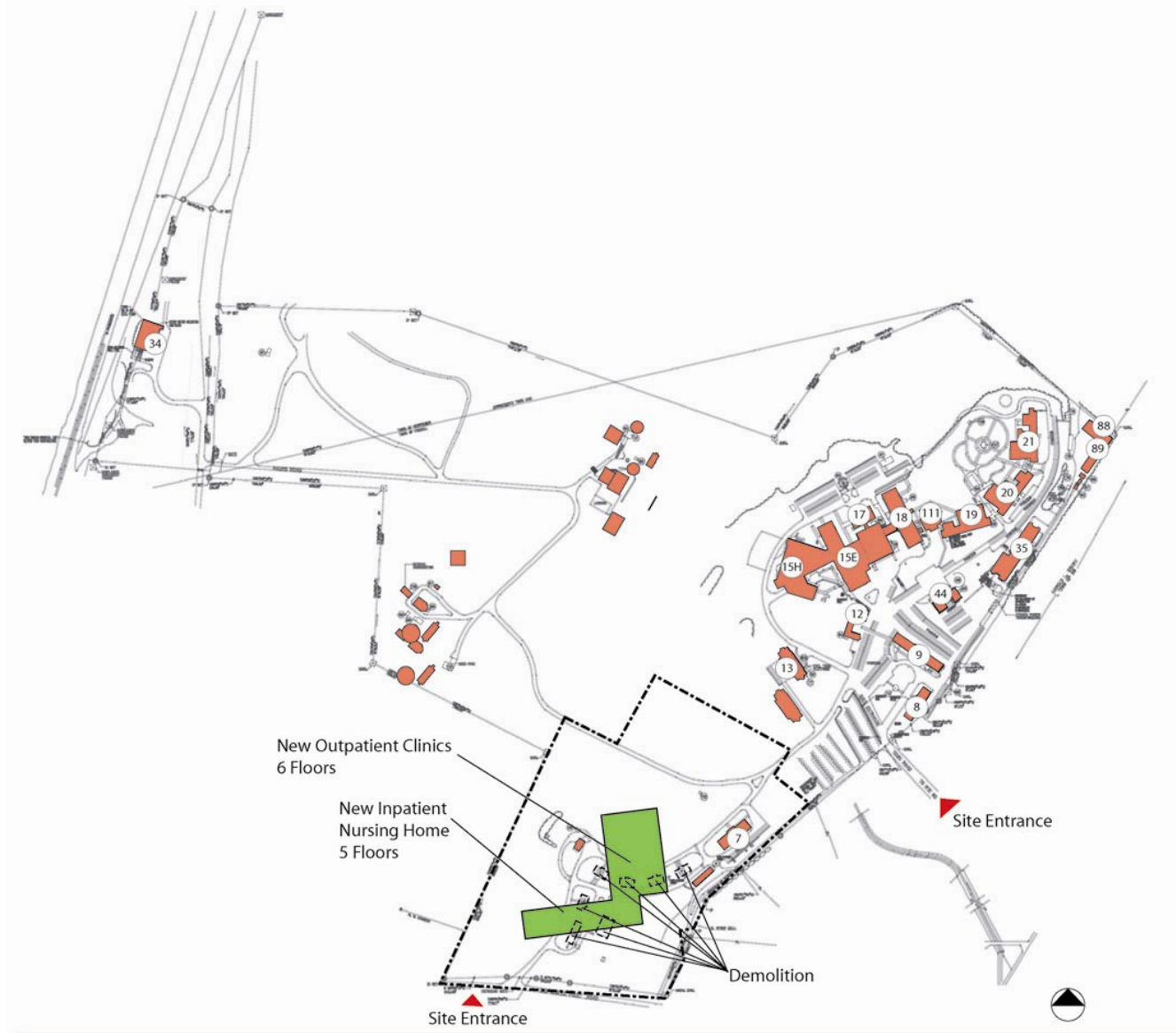
Figure 14: Proposed New Site Plan - BPO 8 (At Castle Point, Construct All New Facilities South of Existing Buildings)
