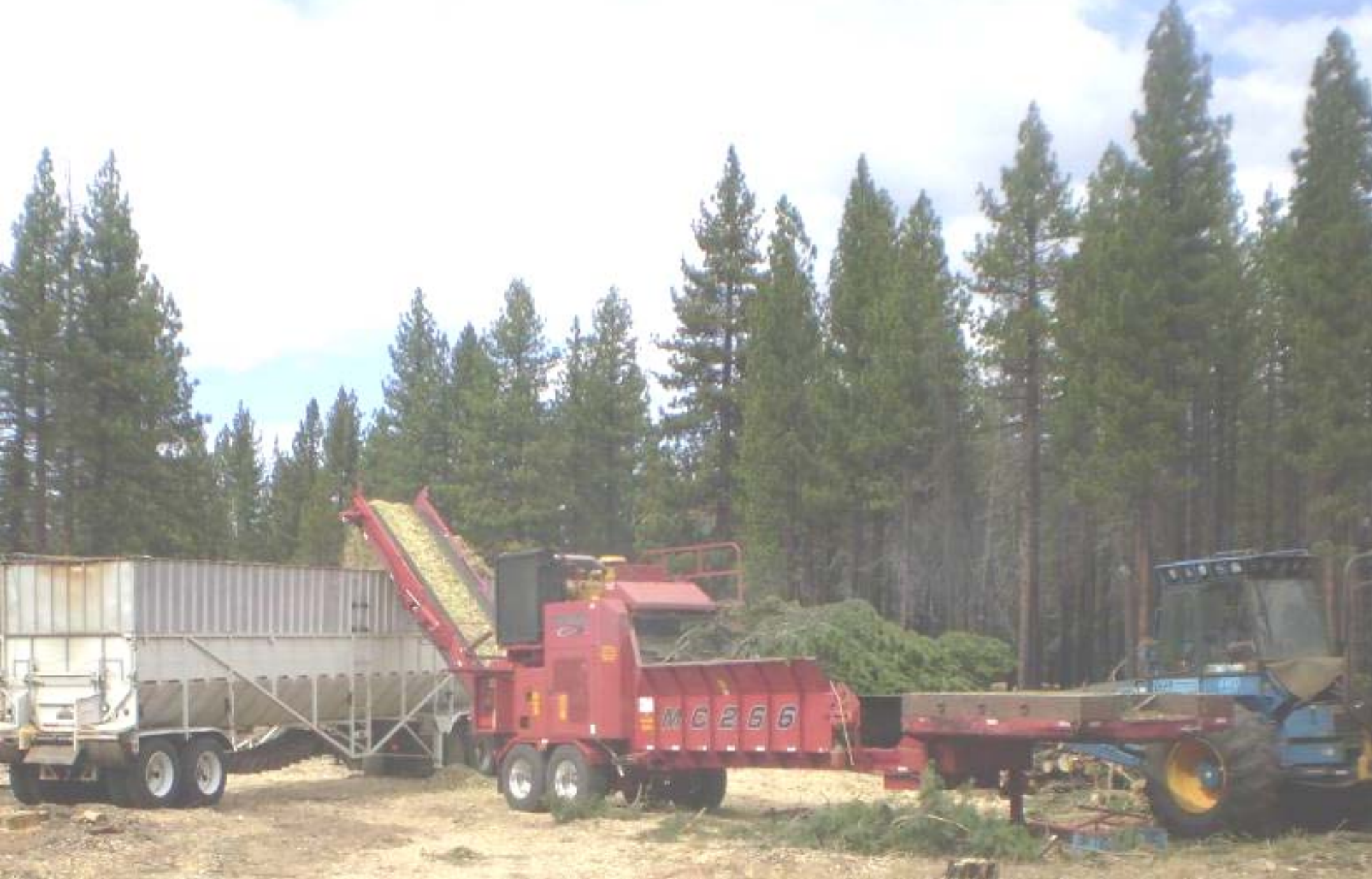
Chipping and hauling of cut material
