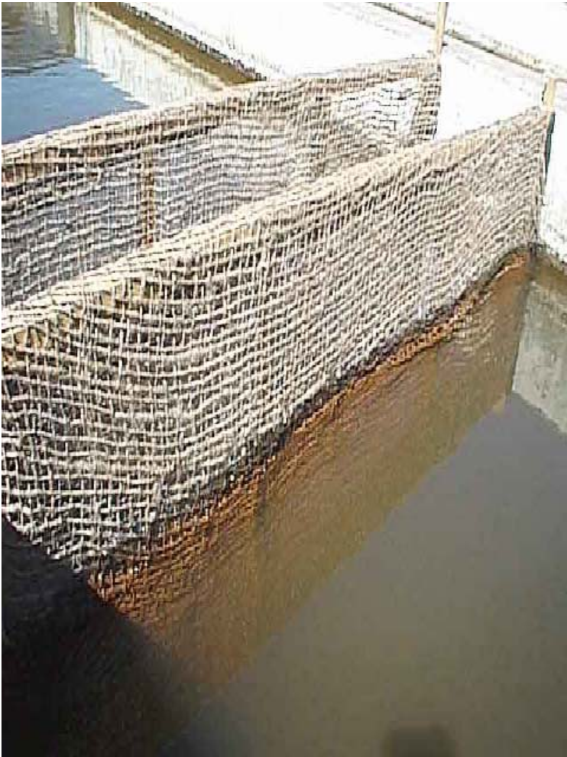
Figure 4 - 3. Particle curtains of woven jute on wood frames (Iwinski, 2004).
