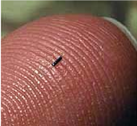
The relative size of a coded-wire tag is apparent when placed on a finger-tip (above). A magnified image can be viewed below.
