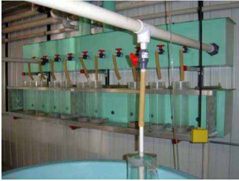
-USFWS The hatching battery at the Genoa National Fish Hatchery, for incubating lake sturgeon eggs, allows multiple hatching jar use as well as isolated hatching into individual tanks.
