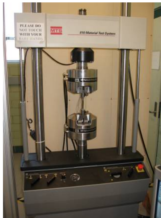
Figure 59. Fatigue test setup.
