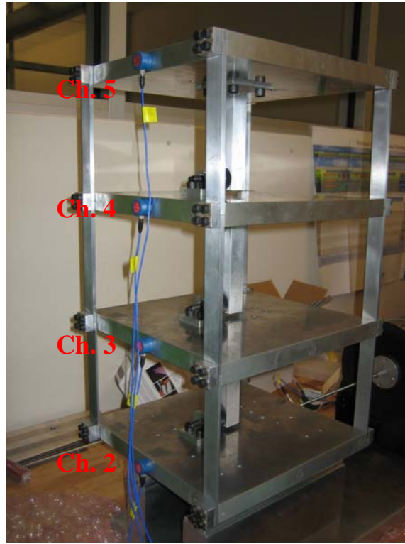
Figure 93. Attachment of accelerometers.
