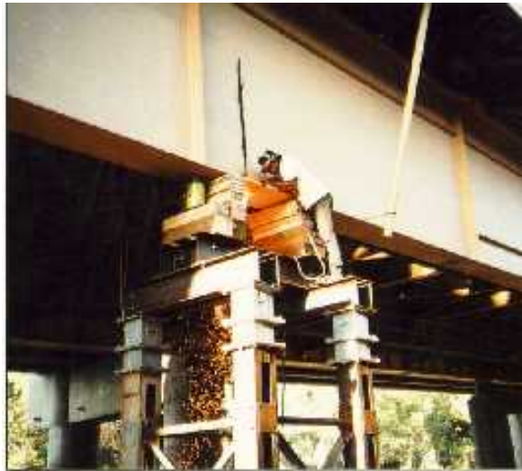
Figure 1. Torch cut that was used to simulate a fatigue crack in a plate girder.
