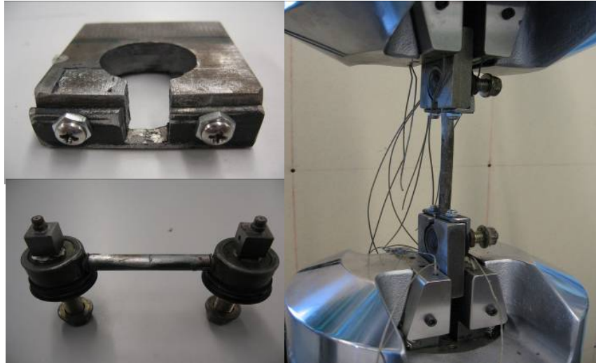
Figure 60. Fixture for placing link under test in fatigue machine grips. Accelerometers attached to the ends of stabilizer bar link.
