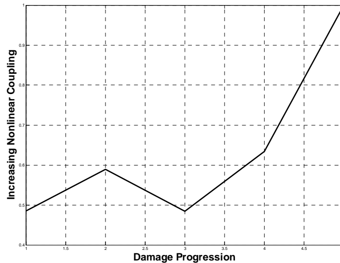
Figure 65. Index based on magnitude of response bispectrum showing progressive increase in nonlinear frequency coupling with growth of fatigue crack.
