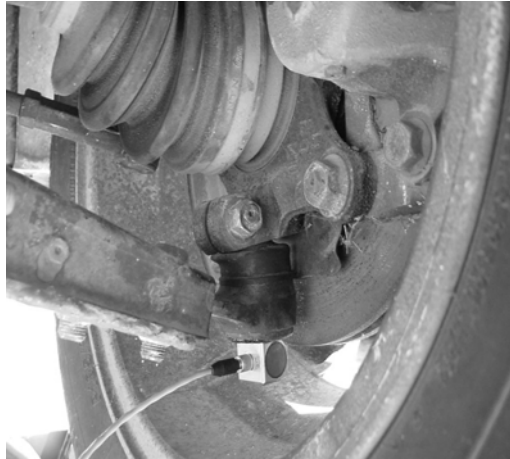
Figure 52. Bolt damage location.
