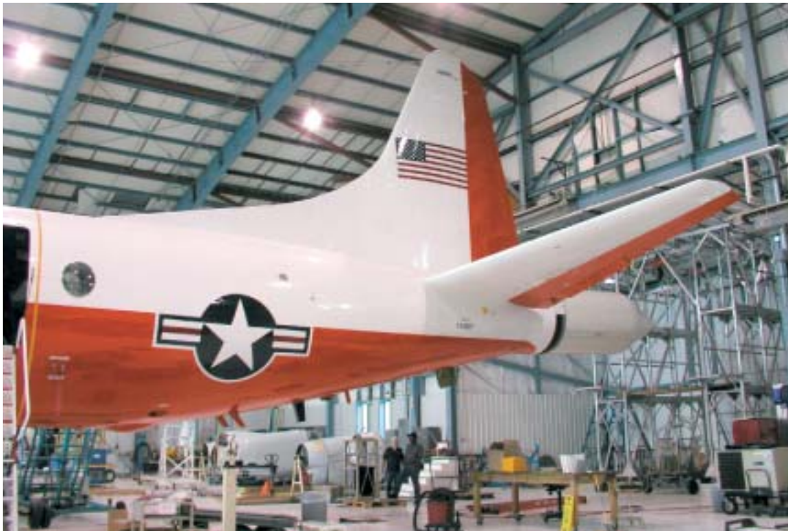
NRL P-3 being outfitted with ELDORA radar at NCAR.
