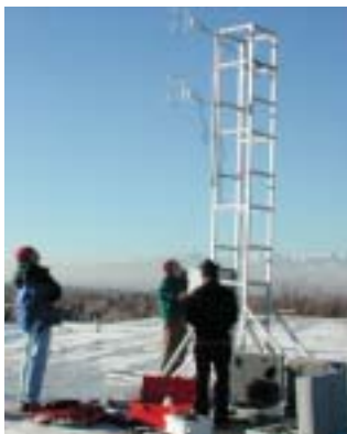
Sonic anemometers installed at Utah elementary school (U. Utah).
