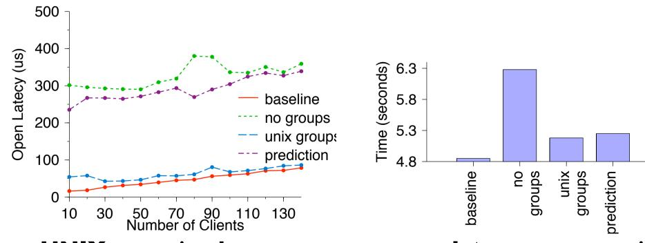
UNIX grouping has an average open latency on par with baseline Ceph. Prediction was unable to make many predictions from IOR2 access patterns and performed worse
