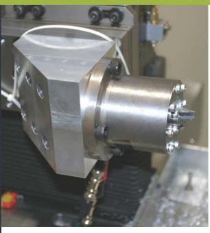
The turning process is very important in many manufacturing applications. In high precision machining, surface finish is strongly correlated with the vibrations and dynamic interactions between the part and the cutting tool. Process characteristics such as spindle speed, cut depth, feed rate, and the part's material properties can vary in real-time with unexpected or undesirable effects on the surface finish of the resulting product.
