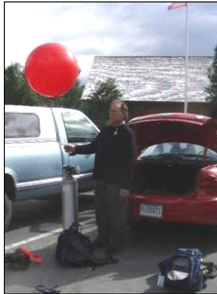
Figure 18. Three-foot diameter red balloon used to evaluate visibility of gravel extraction equipment from key viewpoints at Spencer
