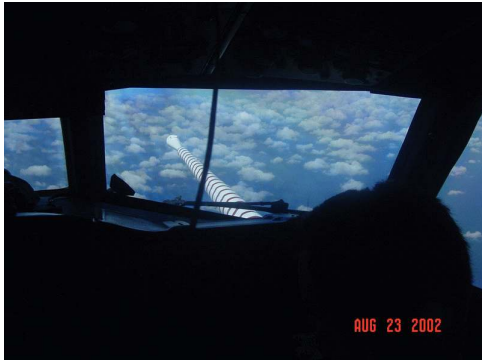
Figure 2. The BAT probe seen from the cockpit of the P3 during a test flight.
