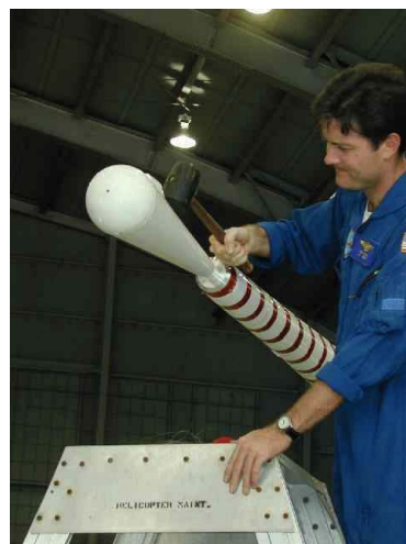
Figure 1. Vibrational testing of the BAT probe on the P3 boom.
