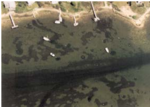
Figure 17. Propeller and mooring chain scour marks near docks (left) and propeller wash scour marks in Waquoit Bay (right). (Photo credit: R. Crawford).
