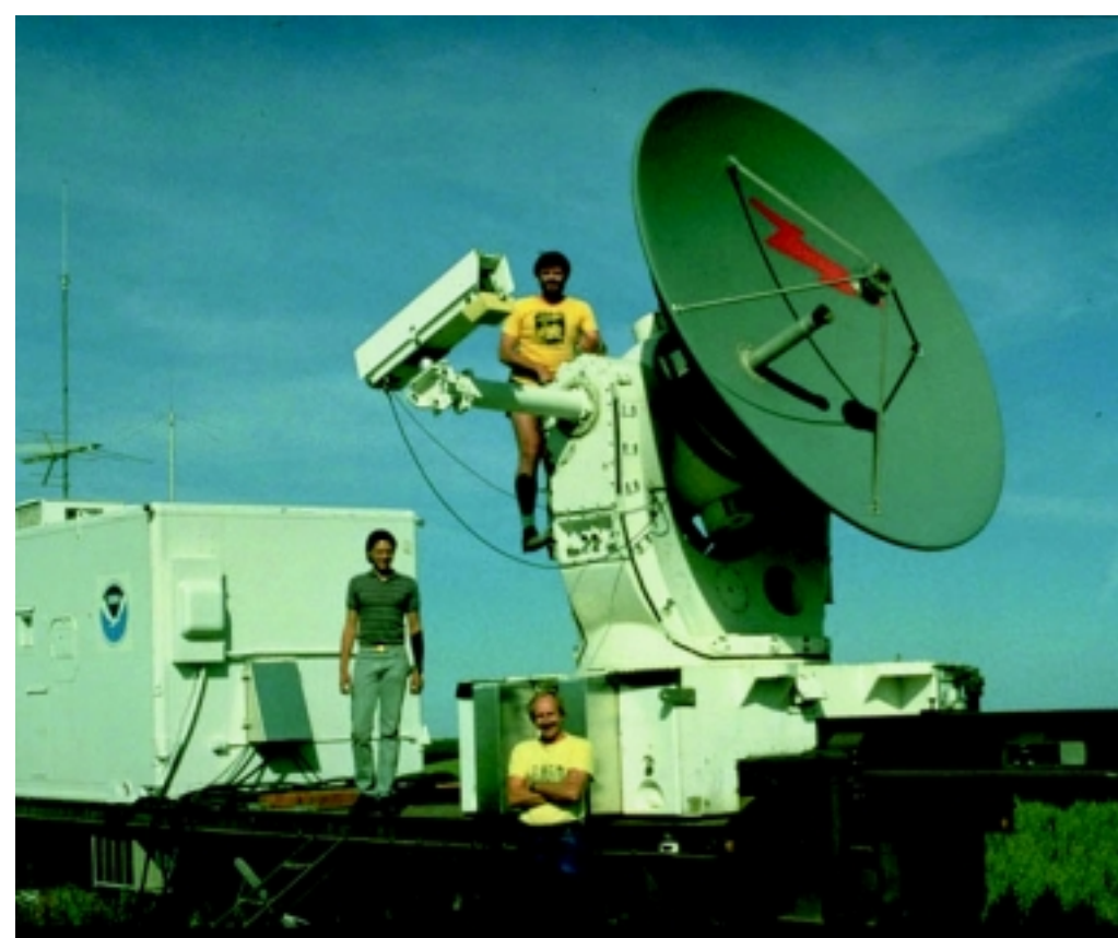
This NOAA radar is used to observe clouds. In the atmosphere, the long-wavelength radar pulses interact with water droplets and ice crystals in clouds.
