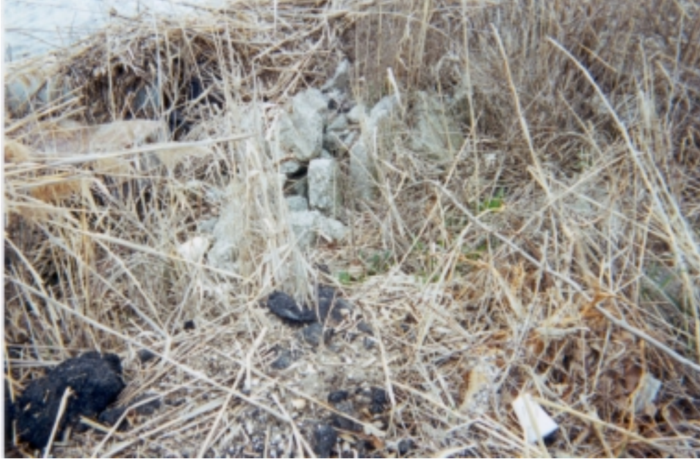
Photograph 8: Close-up of the material that makes up the shoreline. The shoreline is mostly loosely consolidated soils with a significant amount of cobble sized (and larger) rubble.
