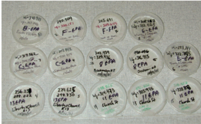
Figure 2. WTC bulk dust samples were size-fractionated by NYU. Filters containing the PM 2.5 fraction were received at the U.S. EPA in Research Triangle Park, NC on 10/26/2001, and were inspected and photographed 10/29/2001.
