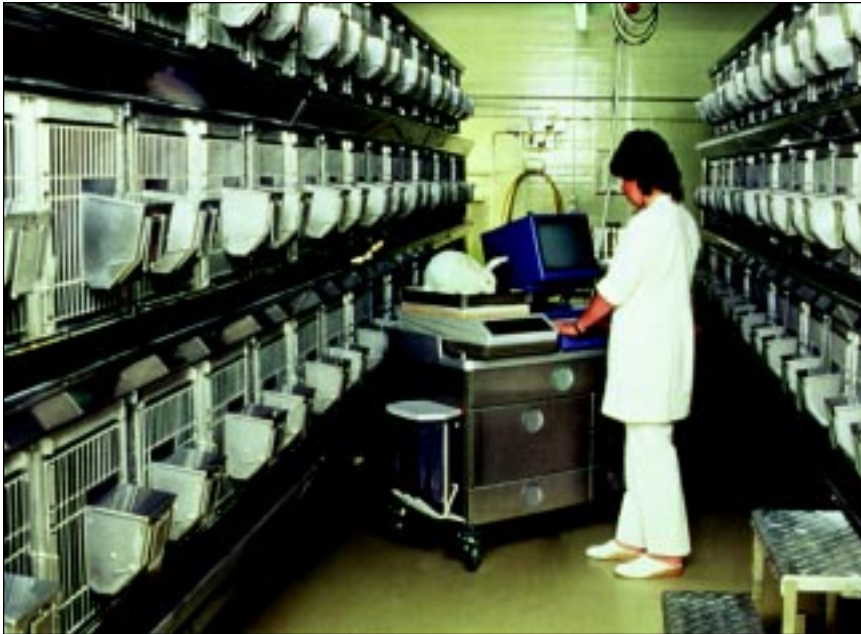
A rabbit is weighed on an automatic scale system that simultaneously enters the weight into a computer.
