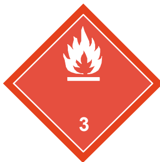
Pictogram for flammable liquid in the UN Model Regulations (Symbol: Flame: black or white; Background: red; Figure 3 in bottom corner; minimum dimensions 100 mm × 100 mm.)
