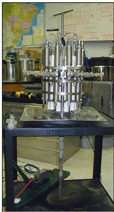
Figure 2: The first pore-water probe with high pressure stainless steel sample chambers and on/off valves. The 50-cm probe tip is visible below the lab cart. Inserting the probe into the sediment required the entire device to be manipulated on the seafloor.
