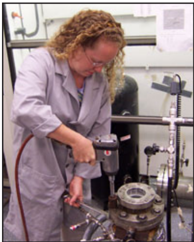
Jennifer Dearman applies some basic engineering technology (a wrench) while assembling a high pressure test cell in the Mississippi State laboratory.
