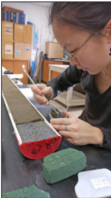
Mea Cook samples a sediment core from the southeast Bering Sea for carbon isotopes and organic biomarker analysis which can give clues to the role of sedimentary methane hydrates in millennial-scale climate change. Photo credit is Tom Kleindinst (WHOI).
