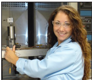
Eilis Rosenbaum with the high-pressure variable volume cell used to form hydrates at NETL in Pittsburgh.
