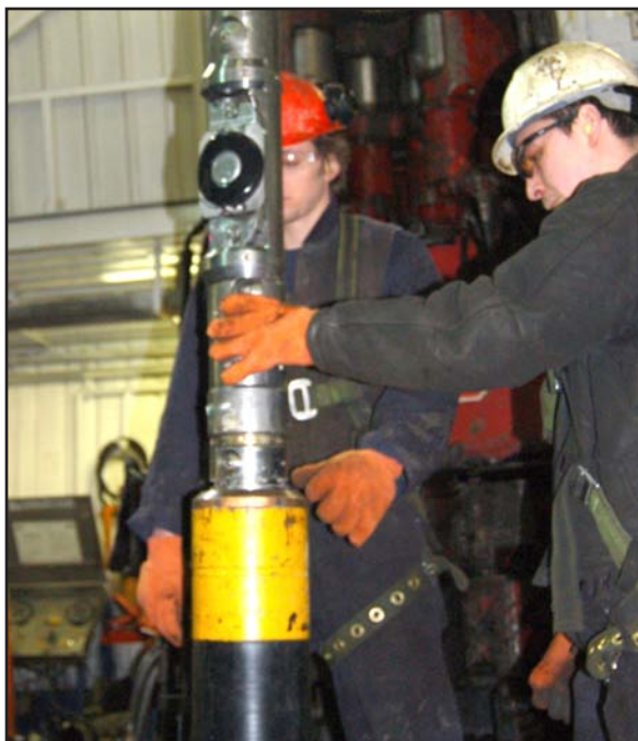
Figure 1: The crew of the Doyon 14 rigging up the Modular Dynamic Tester at the Mount Elbert test site, February, 2007
