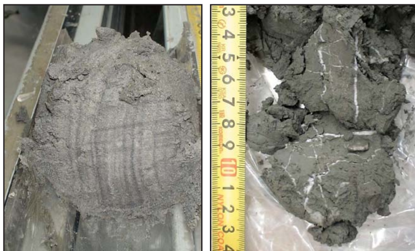
Figure 6: Gas hydrate present in clay material as veins, displacing sedimentary grains, and as a pore-filling matrix within sandy layers.
