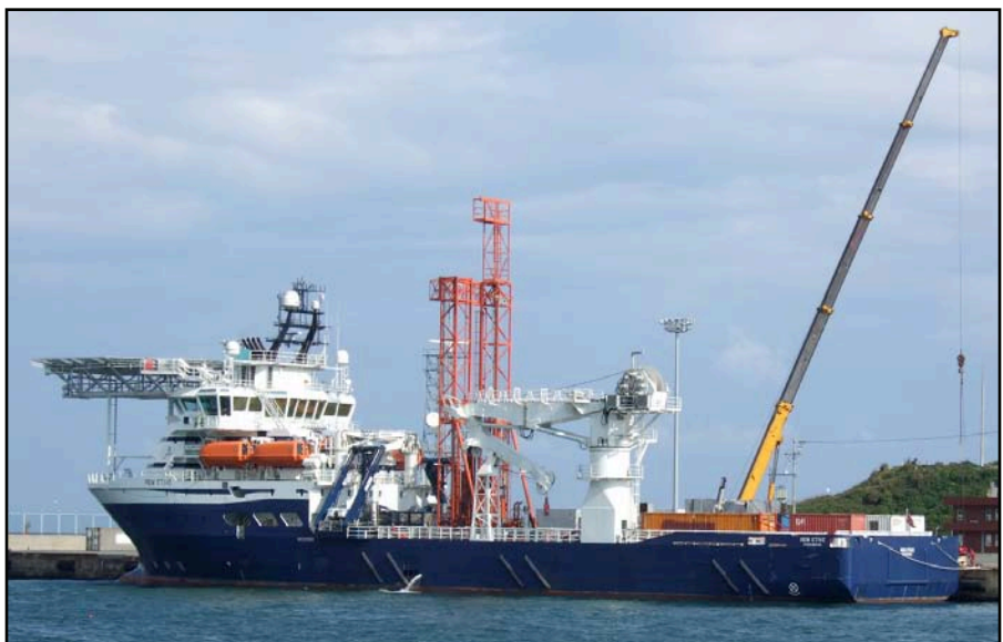
Figure 1: The REM Etive in dock at Busan, Korea, with the R100 drill rig amidships and laboratory containers aft.
