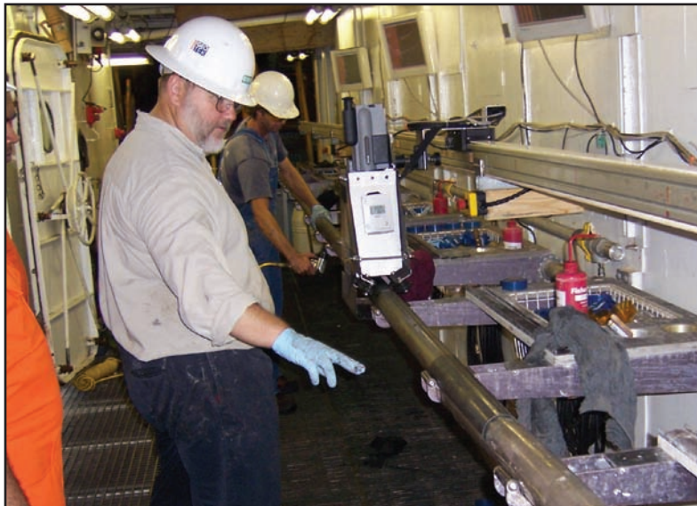
• Science team leader Dr. Timothy Collett guiding core sampling on the catwalk of the JR • (Courtesy NGHP Expedition 01)
