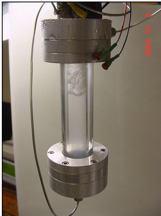
Image of methane hydrate forming in the sapphire vessel at 280 K and 13.8 Mpa.
