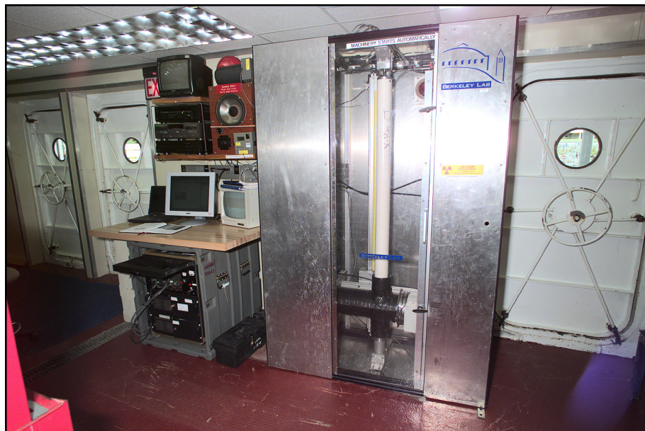
The x-ray CT system installed on the Bridge Deck of the JOIDES Resolution during ODP Leg 210.
