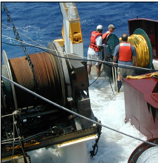
A hydrophone streamer is being deployed from the stern of the R/V Gyre in heavy seas.
