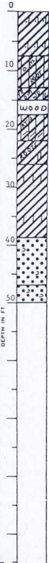
Number in first column indicates number of blows of 140-lb. hammer dropped 30 in. required to seat 2-in. O. D. splitspoon sampler 6 in. Number in second column indicates number of blows of 140-lb. hammer dropped 30 in. required to drive 2-in. O. D. splitspoon sampler 1 ft. after seating 6 in.
