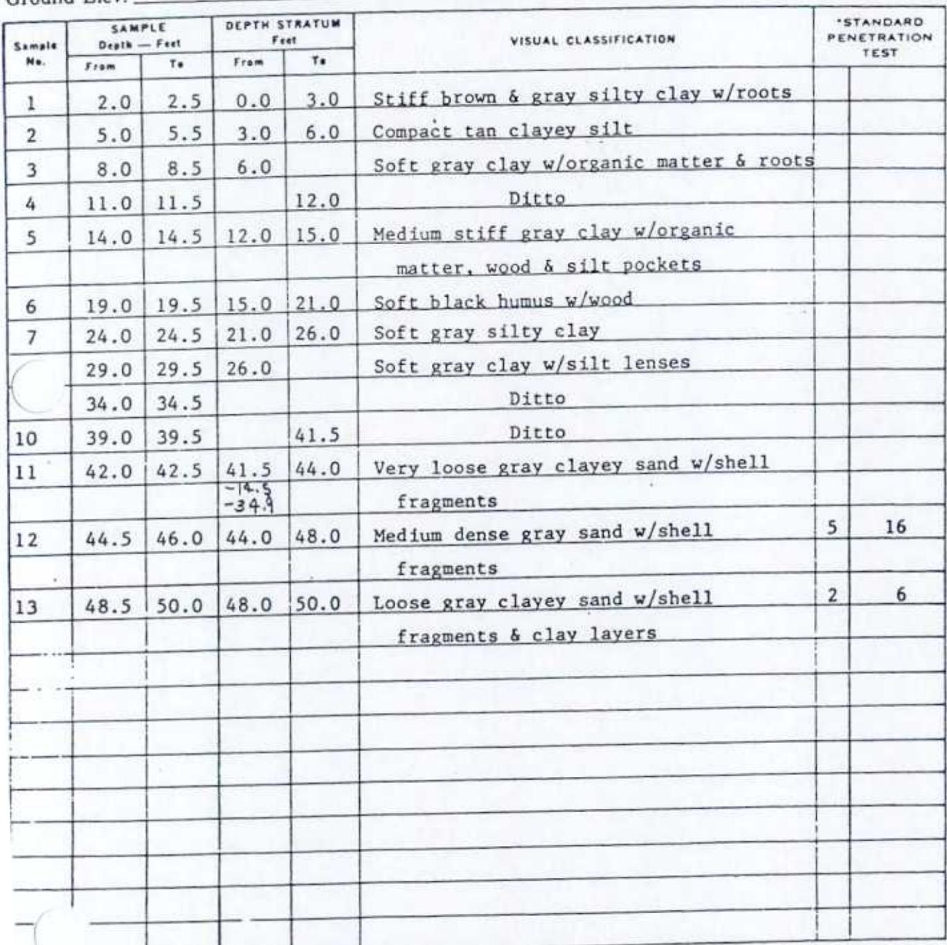
Number in first column indicates number of blows of 140-lb. hammer dropped 30 in. required to seat 2-in. O. D. splitspoon sampler 6 in. Number in second column indicates number of blows of 140-lb. hammer dropped 30 in. required to drive 2-in. O. D. splitspoon sampler 1 ft. after seating 6 in.
