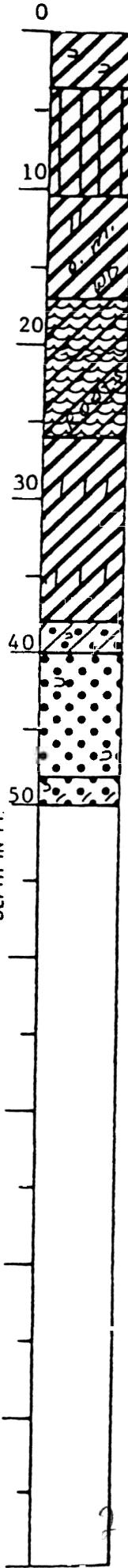
\*Number in first column indicates number of blows of 140-lb. hammer dropped 30 in. required to seat 2-in. O. D. splitspoon sampler 6 in. Number in second column indicates number of blows of 140-lb. hammer dropped 30 in. required to drive 2-in. O. D. splitspoon sampler 1 ft. after seating 6 in.
