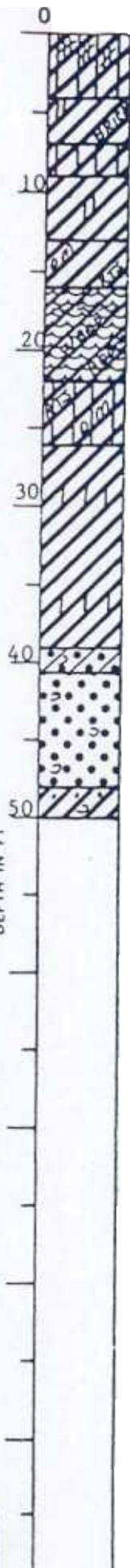
Number in first column indicates number of blows of 140-lb. hammer dropped 30 in. required to seat 2-in. O. D. splitsoil sampler 6 in. Number in second column indicates number of blows of 140-lb. hammer dropped 30 in. required to drive 2-in. O. D. splitsoil sampler 1 ft. after seating 6 in.
