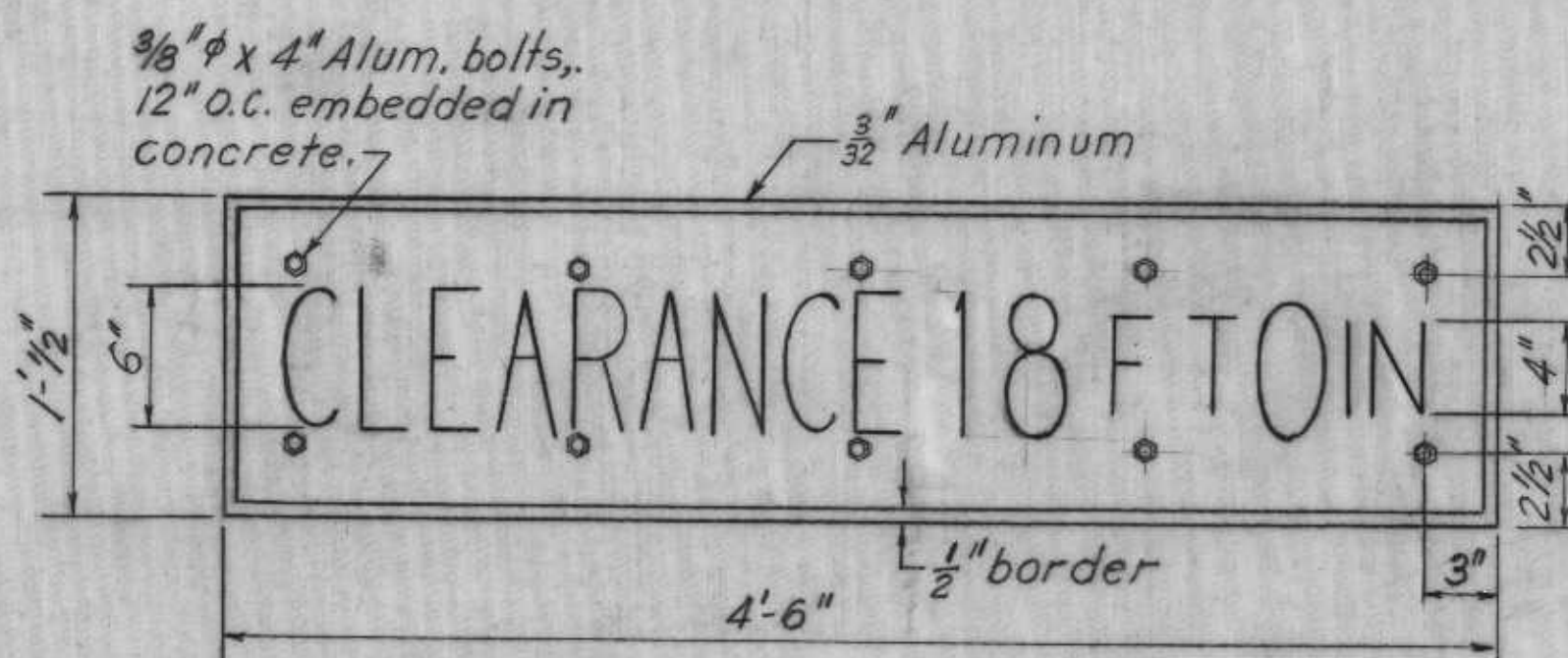
VERTICAL CLEARANCE SIGN Scale: 1 1/2" = 1'-0" Note: Use scotchlight yellow background with 1/4" width block letters. Sign to be put on flood and protected side of removable beams.
