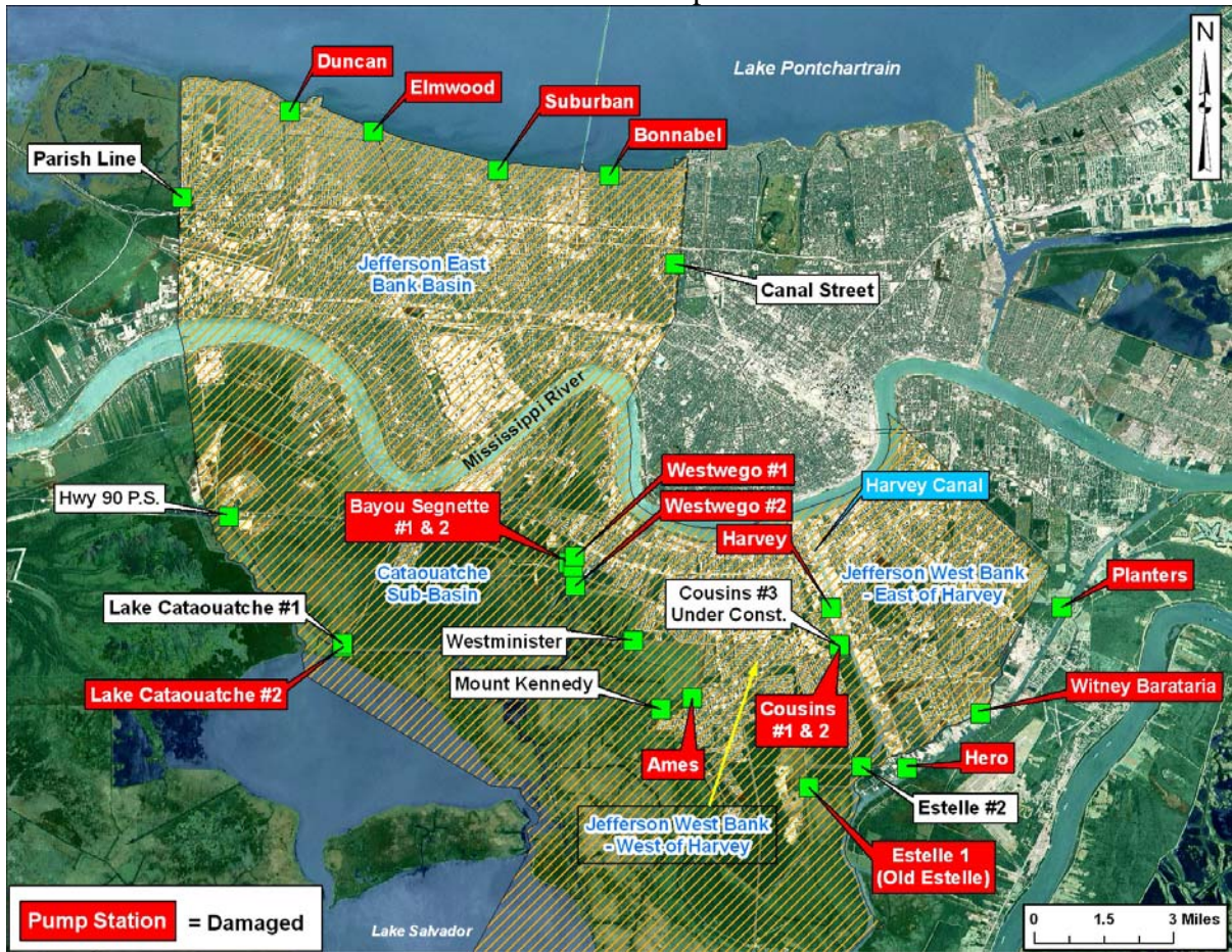
Figure Exec 1. Jefferson Parish Pump Station
