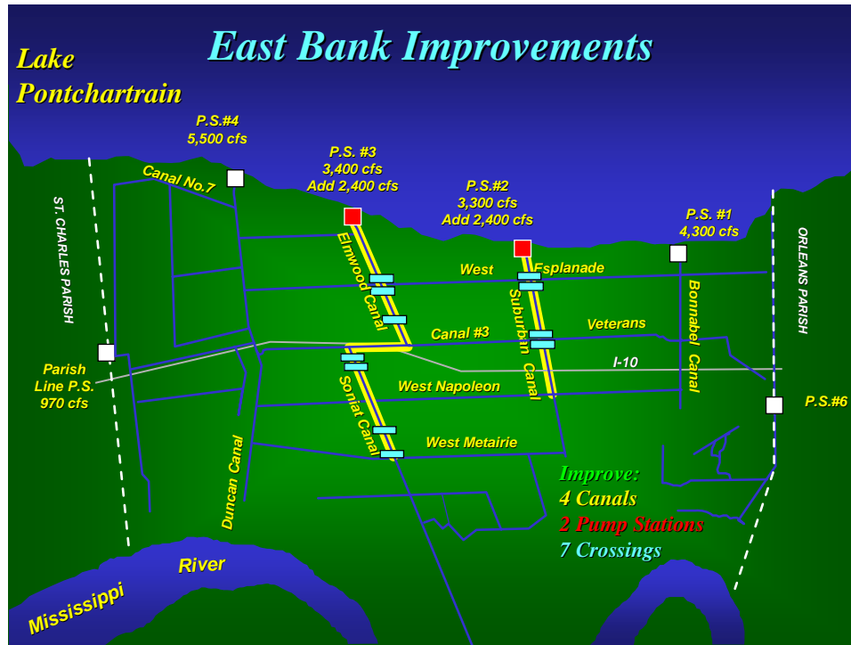
Figure 2. Federal (SELA) East Bank Basin Improvements
