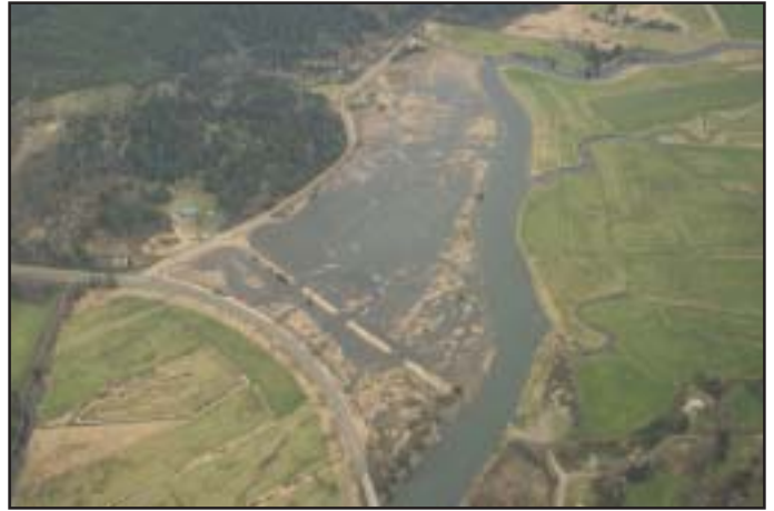
At the Nestucca Bay National Wildlife Refuge in Oregon, the FWS worked with multiple federal, state, tribal, and local agencies, as well as with conservation groups and a private foundation, to remove dikes and thereby restore 82 acres of estuarine wetlands benefiting migratory birds, salmon, and other species. (FWS)
