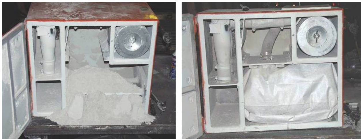
Figure 5. Dust as normally deposited in the collector box (left) and the collector box with bag utilized (right)
