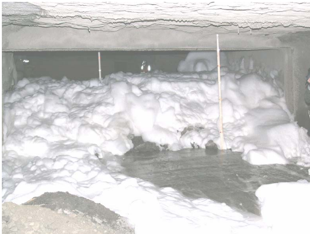
Figure 7. Movement of foam around first crosscut in B drift during experiment 1.
