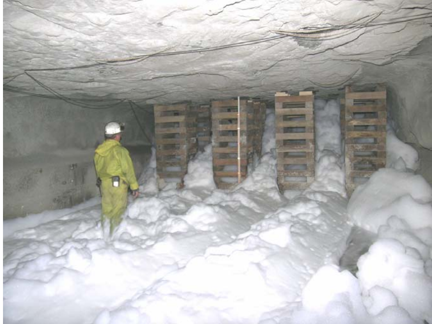
Figure 9. Foam behavior at crib blocks in A drift.
