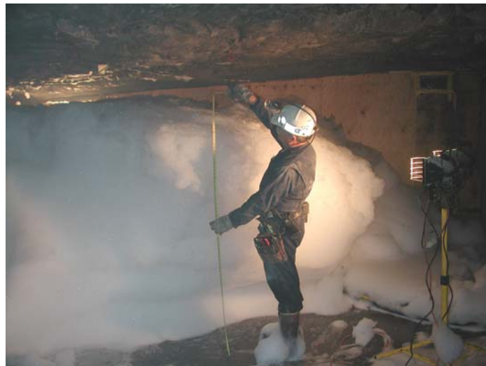
Figure 20. Researcher measuring the height of the foam plug in E drift.
