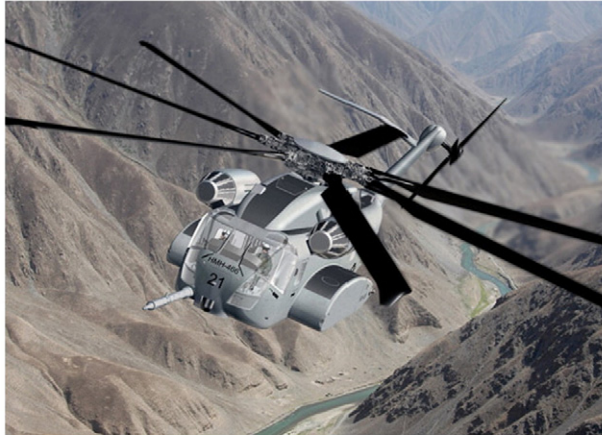
The CH-53K helicopter's maximum gross weight will increase to 84,700 pounds, versus 73,000 pounds for the CH-53E. It is being designed to carry a cargo load of 27,000 pounds (13.5 tons) 110 nautical miles, operating at an altitude of 3,000 feet and an ambient temperature of 91.5 degrees Fahrenheit. This is nearly double the capacity of the current CH-53E Super Stallions.
