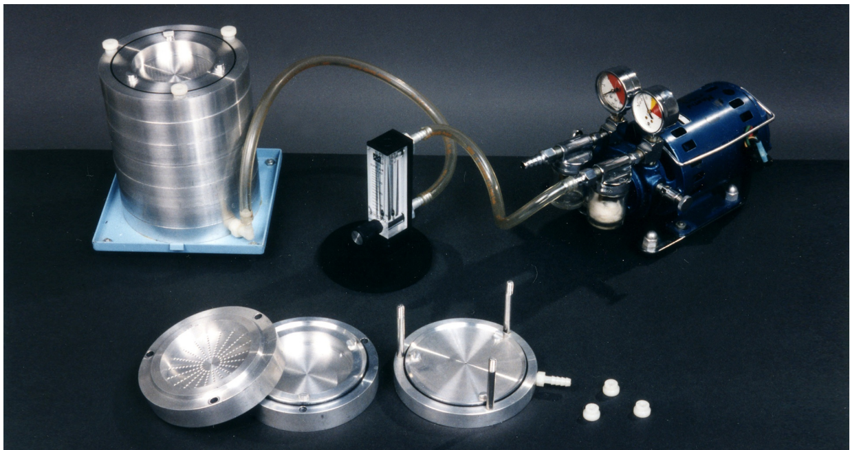
Figure 5. A 2-stage (foreground) and a 6-stage Andersen sampler. A 6-stage Andersen sampler properly connected to a flowmeter and a vacuum pump (background).
