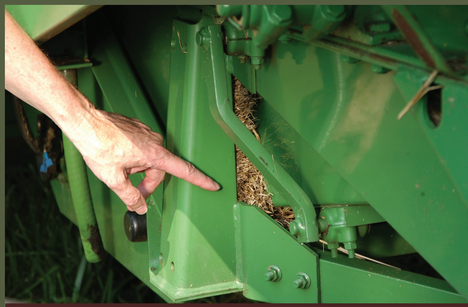
Plant material remaining within crevices of machines can violate field release conditions. Proper cleaning can help prevent the spread and establishment of regulated GE material.
