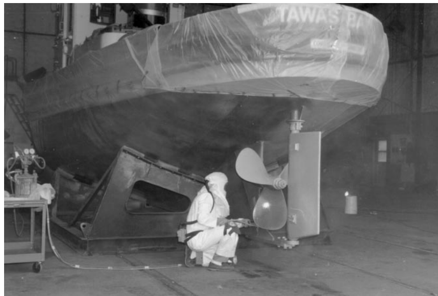
Figure 1. Applying the compound to the Tawas Bay
