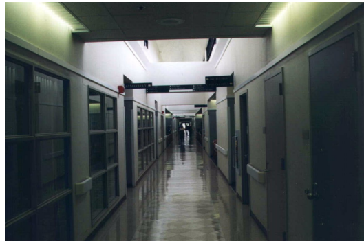
Perpendicular lighting to "shorten" a long corridor.
