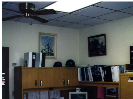
Residential fan unnecessary if mechanical system is well designed.
