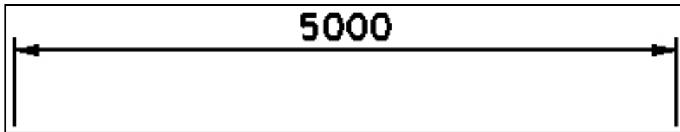
Figure 3-9. Proper dimension presentations for metric measurements with four or fewer digits
