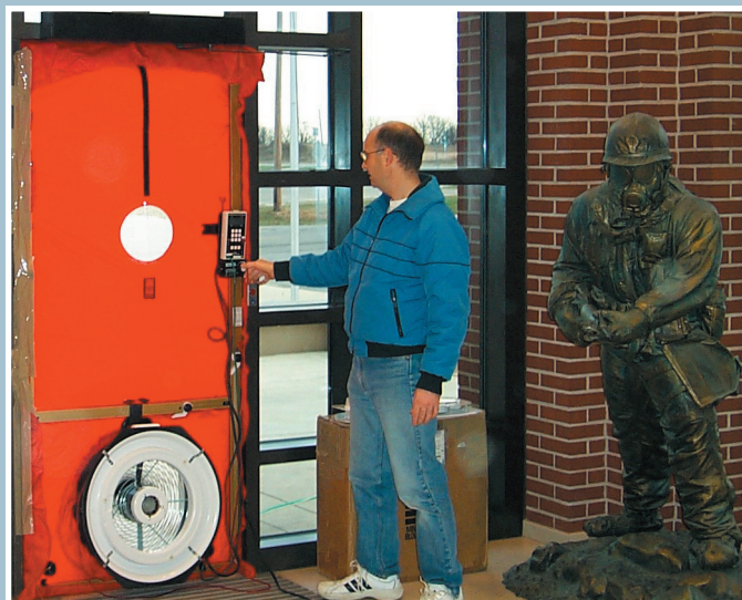
Blower Door Test - Leakage rate testing for facility collective protection against chemical/biological threats.
