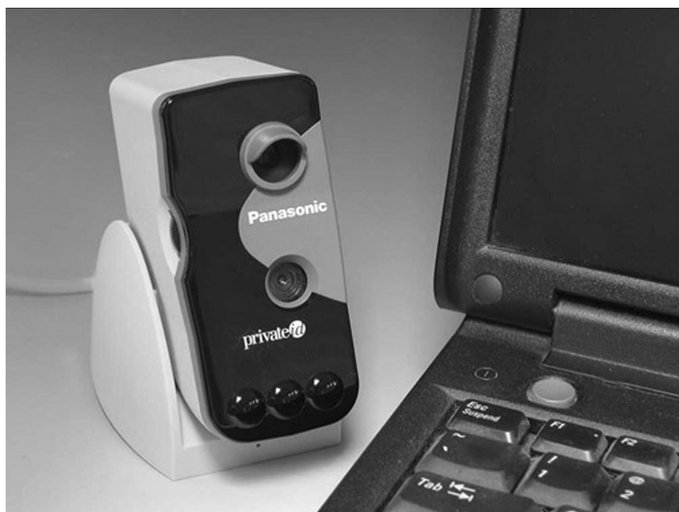
Figure 14: A Desktop Iris Recognition System
