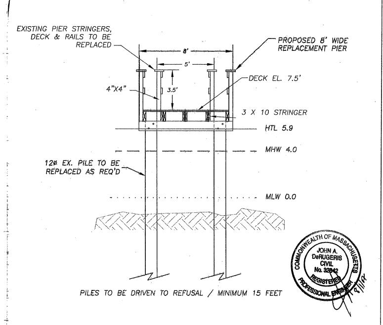
URPOSE: PROPOSED PIER RECONSTRUCTION AND FLOAT EXPANSION WILL IMPROVE ACCESS O NAVIGABLE WATERS DATUM: MLW = 0.0MHW = 4.0
