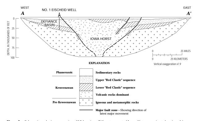
**Figure 2.** Schematic geologic cross section of Midcontinent Rift system, central Iowa. Note approximate location of Amoco M.G. Eischeid No. 1 well with respect to Iowa horst. Line of section is shown in figure 1. Modified from Palacas and others (1990).
