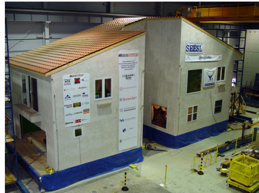
Figure 4. NEES shake table testing of a full-scale wood frame, residential building. © 2006 by Andre Filiatrault.
