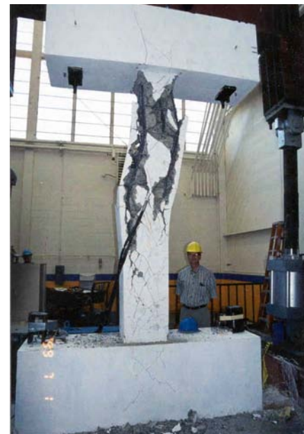
Figure 16. Laboratory testing of an older concrete column design. This type of damage is similar to that seen in Figure 2. © 2002 by Pacific Earthquake Engineering Research Center.
