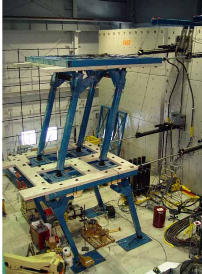
The NEES Nonstructural Component Simulator. Image courtesy of the University at Buffalo's Structural Engineering and Earthquake Simulation Laboratory (SEESL).
