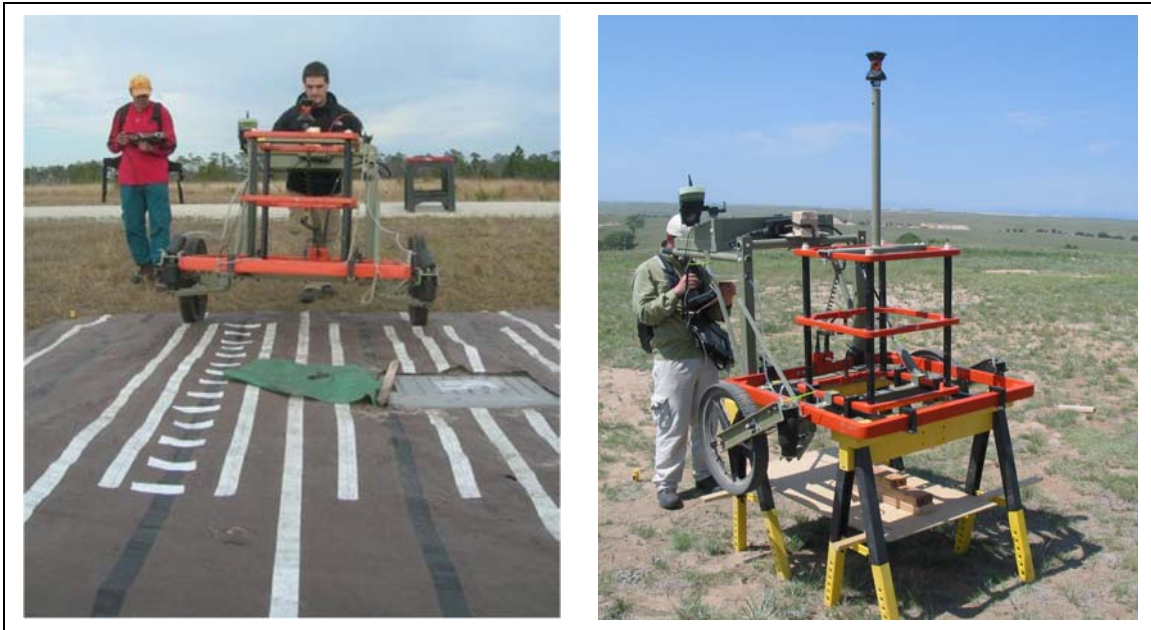
Figure 5. Tarpaulin with marked lanes for cued interrogation (on right) and the EM-63 collecting calibration data while on two plastic sawhorses (on left).
