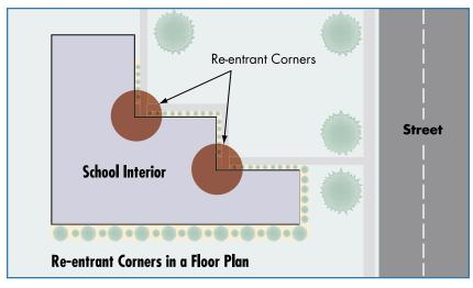
Figure 3-1 Re-entrant corners in a floor plan SOURCE: U.S. AIR FORCE, INSTALLATION FORCE PROTECTION GUIDE
