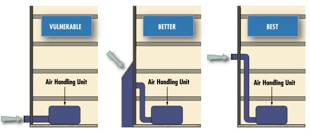
Figure 3-7 Example of protecting outdoor air intakes
