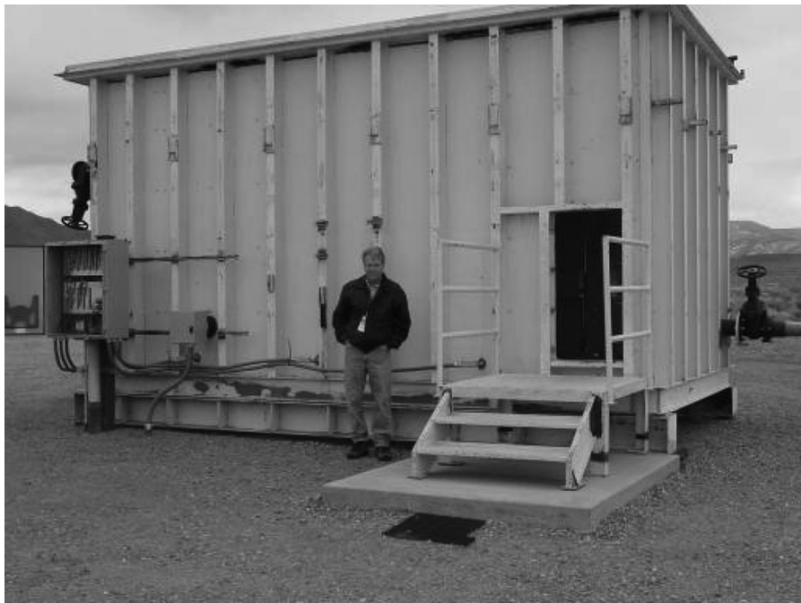
Fig. 2. Aerosolization chamber—stainless-steel chamber with a capacity of 0.06 kg of high explosive (Harper et al. 2006).
