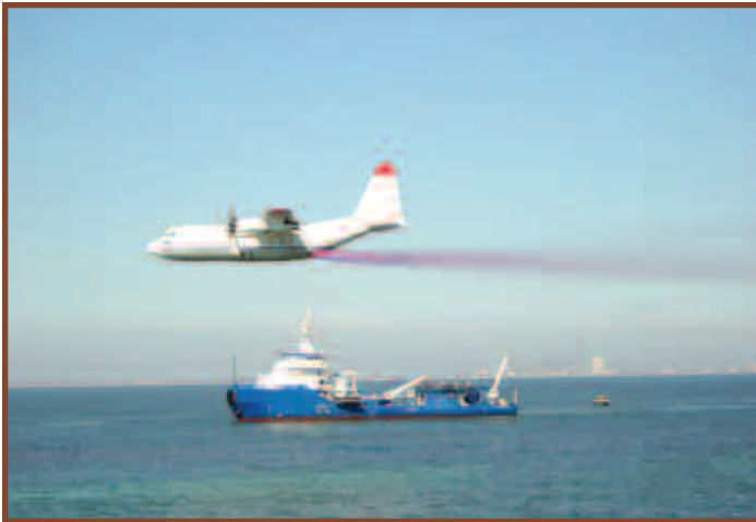
A C-130 Hercules leased by the Marine Spill Response Corporation drops dyed water on a simulated oil slick. An Air Force C-130 also took part in the demonstration, which tested the ability to drop dispersants from aircraft to break up offshore oil spills.
