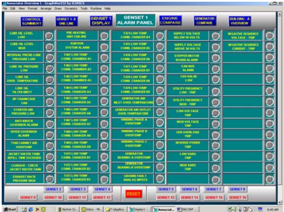
Figure 28: Generator Annunciator Display
