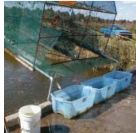
Emptying fish trap to evaluate fish passage effectiveness at Mattamuskeet NWR, NC.
